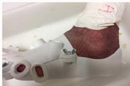
Figure 3: Glove printed in Polyamide 12.
