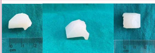
Figure 2: Post-tibial polyethylene fracture piece that removed during the operation.
