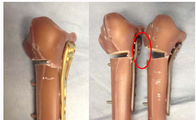
Figures 4 and Figure 5: Loss of reduction without bending of the plate on the left Synthes® plate; bending of the Stryker® plate.
