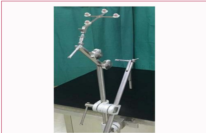
Figure 2: Arm with two grippers for the tracker devices was fixed to the side bar of the operating table. (1) Tracker for coronal plane and axial plane. (2) Tracker for sagittal plane.
