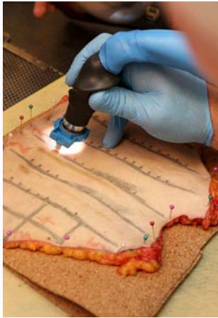
Figure 3: Photo showing the application of the plasma to the sample. The waypoints used to control the speed can be seen as well as the demarcation between tracks which received differing exposure levels.
