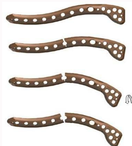
Figure 6: Schematic representation of the process of plate fracture from the superior (left) and postero-anterior views (right). Primarily, mechanical loads acting on the distal part of the plate resulted in brittle fracture of its posterior branch, than anterior one.
