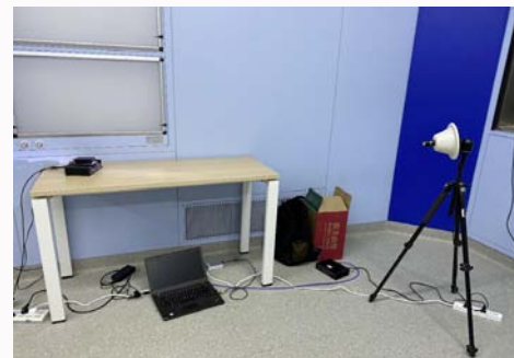
Figure 2: VLC video transmission system used in the digital operation room.
