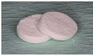
Figure 1: Photograph of OCP/Col discs, which are 9 mm in diameter and 1.5 mm thick. The weight percentage of OCP granules in OCP/Col was 77%. OCP/Col has almost 92% porosity and bimodal peaks of 48 \mu\text{m} (main pores) and 0.3 \mu\text{m} (minor pores), and its specific surface area (SSA) was 17.8 \text{m}^2/\text{g} .
