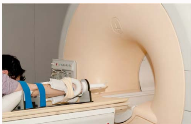
Figure 2: Jig prototype in use in an MRI machine with wrist coils attached.
