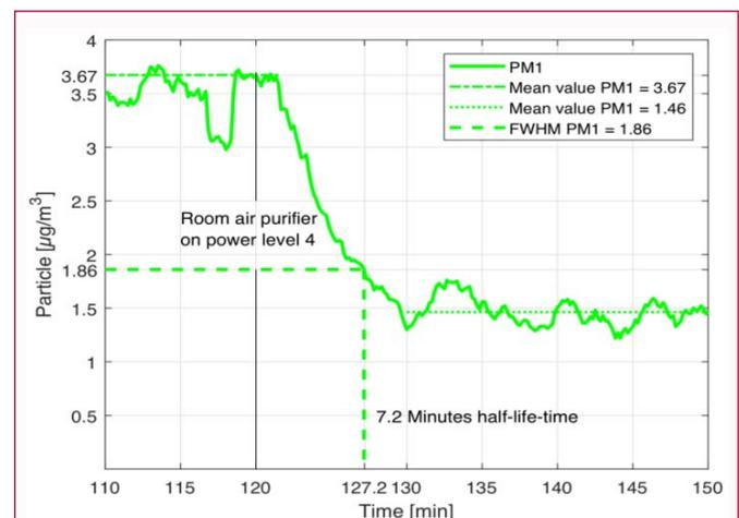
**Figure 1:** Aerosol concentration ( $\text{PM}_{1.0}$ ) from minute 110 to 150. Minute 120 marks the start of the air filter system at Full power. Half-time reduction was achieved after 7.2 min.
