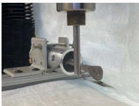
Figure 4: Biaxial load frame applying load to sawbones specimen during torsion test.
