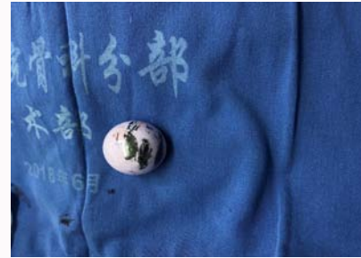
Figure 3: The ceramic femoral head removed from the patient. The bearing surface had worn severely.
