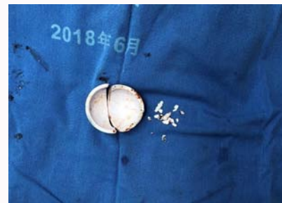
Figure 4: The ceramic liner removed from patient. The fragmented edge of the liner had detached from the acetabular component and the small debris from the fragmented edge were removed around the joint.
